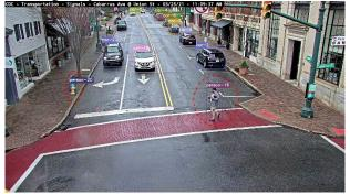
(c) A fire hydrant detected as a pedestrian and a pedestrian using a phone while crossing the road
