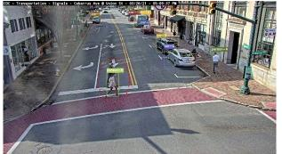
(g) An occluded and non-detected pedestrian crossing the road Figure 7. Challenges in pedestrian and vehicle detection and tracking
