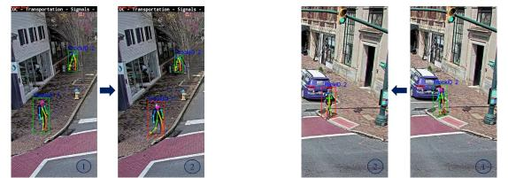
Figure 8. Illustrations of pedestrian crossing intention estimation. (a) Crossing from the left sidewalk (b) Crossing from the right sidewalk
